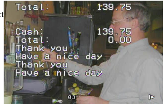
Illustration 1: Text Inserter from a POS on to CCTV Video.
