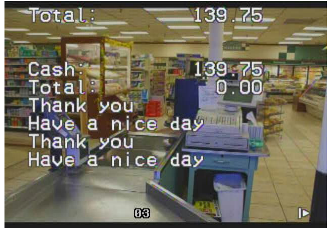
Illustration 7: A Transaction Inserted onto CCTV Video
