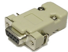
Illustration 2: VRX Loop Back Adapter
